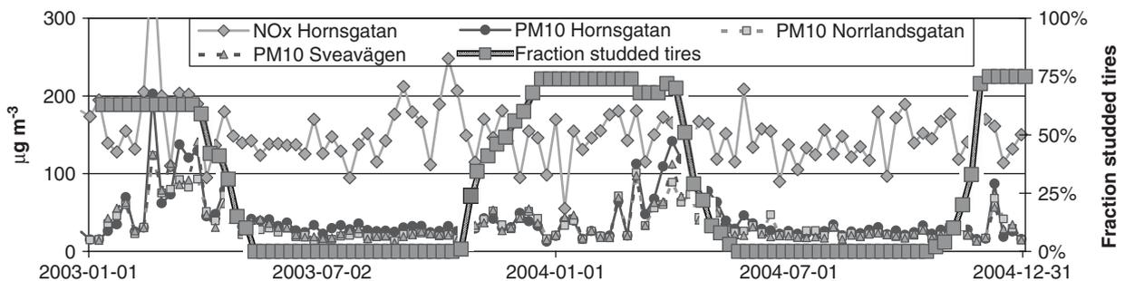
Fig. 1. Weekly average PM<sub>10</sub> and NO<sub>x</sub> levels together with the fraction of studded tyres on light duty vehicles in Stockholm City.
