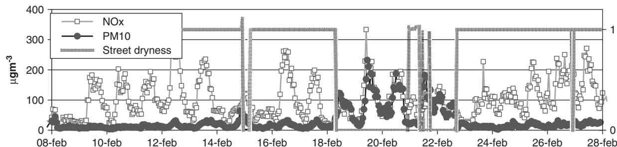
Fig. 2. Observed PM<sub>10</sub>, NO<sub>x</sub> and street wetness at Norrlandsgatan during February 2004. The street sensor signal is one during wet street conditions and zero during dry conditions.
