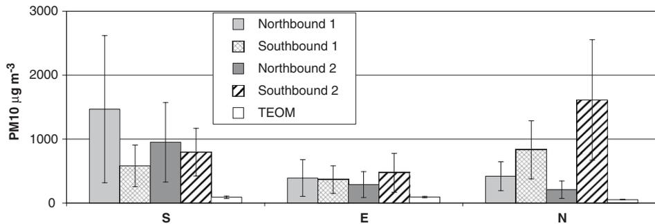
Fig. 6. The average PM10 concentrations along the highway 20 m behind a car that is driving in the verge of the highway. The driving speed for northbound 1 and 2 were 70 and 90 km h<sup>-1</sup>, respectively, and the same for southbound 1 and 2. The vertical bars represent the standard deviation. “S” denotes the untreated stretch, “E” the washed stretch and “N” the CMA treated stretch.
